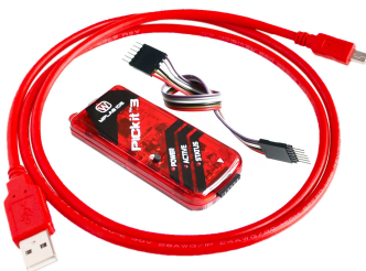
[2474]Programador Pickit 3 Pic Kit 3 Microchip Pic18 Pic32 Pic16 + Pinza + Cable. Bios Eeprom 24
